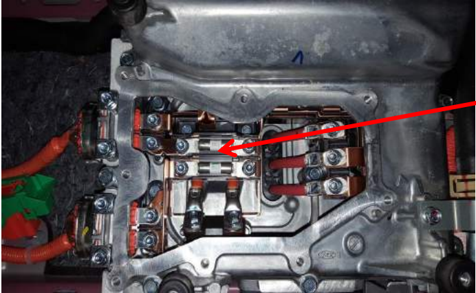
40Amp @300 volts fuses for supplementary Heating system
