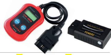
02 MAXISCAN MS300 DTC READER 03 OBD BLUETOOTH ADAPTER
